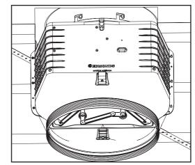
Ensure that the controller is facing towards the low end of the roof and that the cables are routed through the cable slot.
